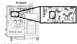
Fig 5. SW 1 Button on PC Board
